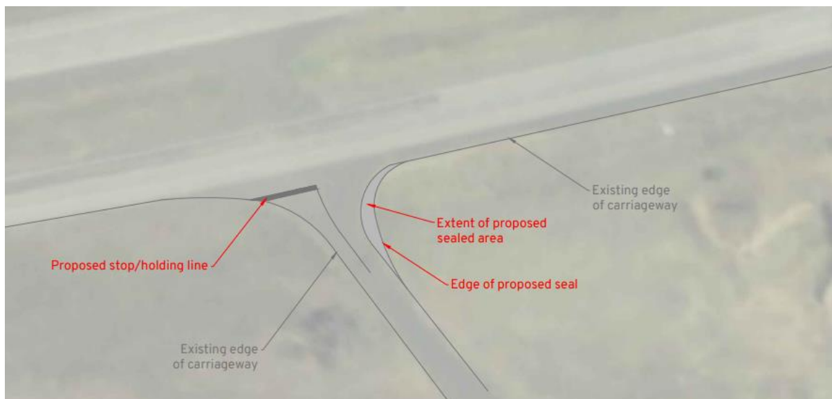
Figures: Hume Highway intersection upgrade plans showing the proposed road upgrades, including sealing, line marking and signage (reproduced from TIA).
